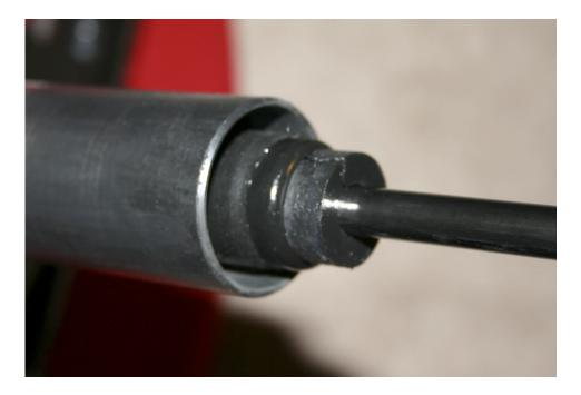
4) Cut a length of copper pipe approximately 10 cm in length (you can go a cm higher or lower, depending on your height preference). Slip that over the shaft and reassemble the chair. No more sinking feeling.
